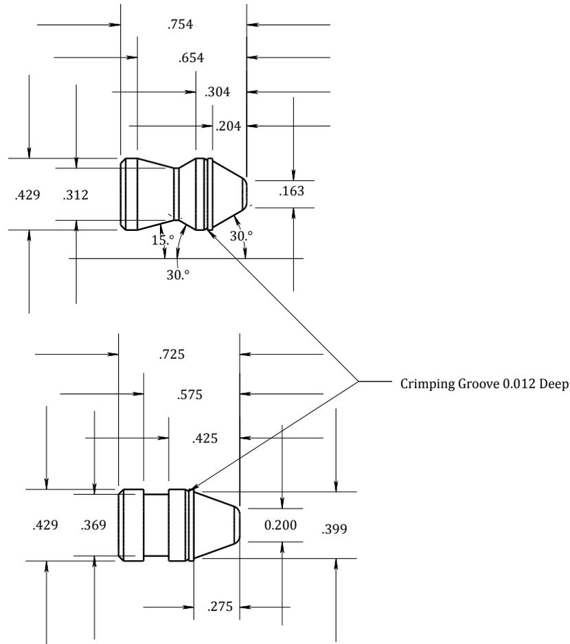
**Figure 4: Design dimensions of my custom double-taper (top) and tapered flat-point (bottom) bullets.**
