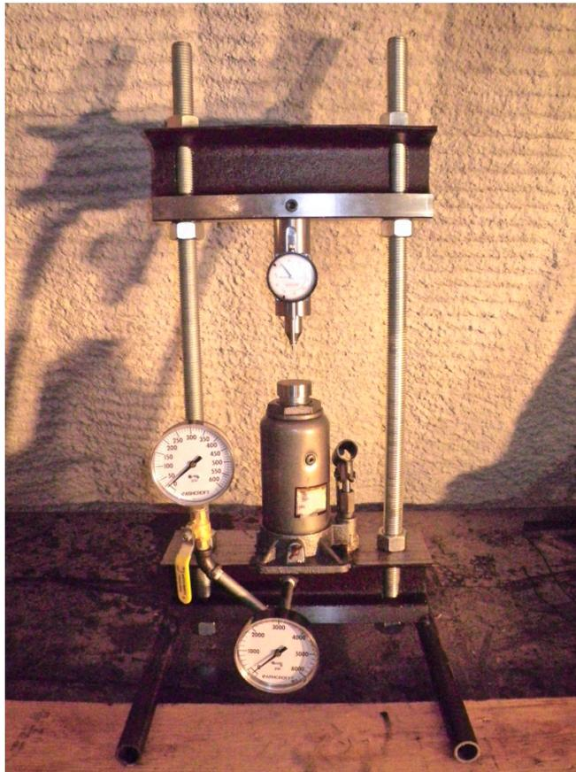
**Figure 1: Photograph of my homemade hardness testing machine, consisting of a hydraulic press with pressure gages to measure applied force and a hardness testing jig mounted at the top of the press.**
